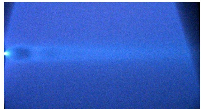
Fig. 7 Helium jet in an Argon medium: highly underexpanded jet, maximum Mach number = 16 , stagnation/ambient pressure ratio p_0/p_a = 304 , density ratio after the normal shock \sim 0.15
