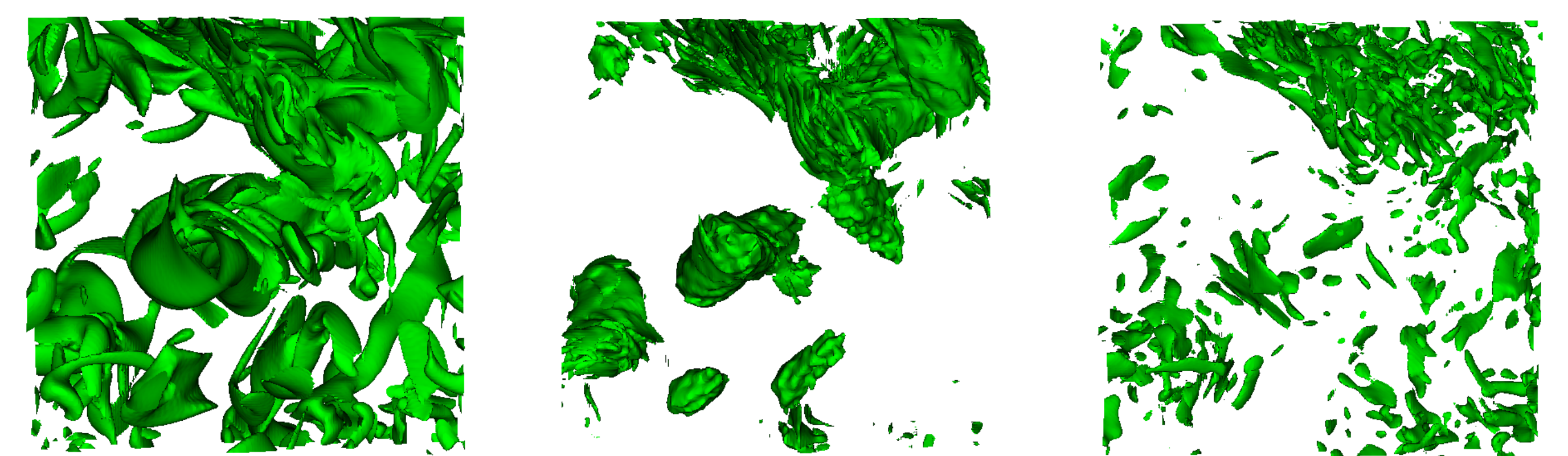
Isotropic Turbulence. Visualization of a component of vorticity, in a three-dimensional cubic domain, 256^3 grid points at Re\lambda=280 , u_{rms} = 0.03684 m/sec (root-mean-square velocity), \nu = 1.5 \times 10^{-5} m 2 /sec (viscosity) and L = 2 m (integral scale). The value of the field is dimensional and is equal to 18. Left: unfiltered field. Center: the wave number range 30-150 is filtered out. Right: the wave number range 30-150 is filtered out.
