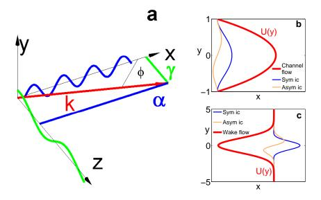
Figure 1: (a) Perturbation geometry scheme. The perturbation propagates in the direction of the polar wavenumber,  $k=\sqrt{\alpha^2+\gamma^2}$ .  $\phi$  is the angle of obliquity with respect to the basic flow. (b)-(c) Symmetric and antisymmetric initial conditions in terms of the perturbation transversal velocity,  $\hat{v}(y,t=0)$  (thin curves), and base flow velocity profiles, U(y) (thick curves).
