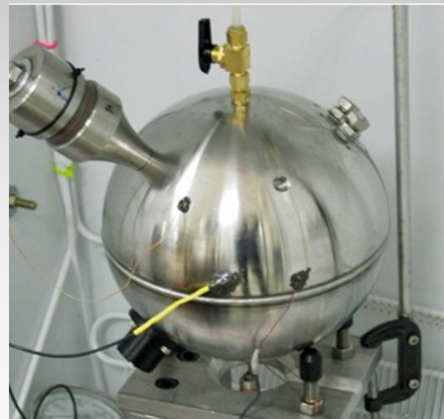
Fig. 1. Schematic of a typical experimental configuration and a photograph of a 9.5-in. windowed resonator used for experiments with a high-speed camera (top right).
